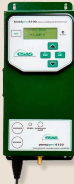
A 'bubbler' or 'gas-purge' water-level instrument, such as the Levelpro 6150 (pictured), is well suited to groundwater monitoring, as no sensitive equipment needs to be underwater. Just lower a simple plastic tube, through which compressed air is bubbled. The pressure on the gas from the weight of water is measured by a sensor above ground, and converted into a water level reading.
