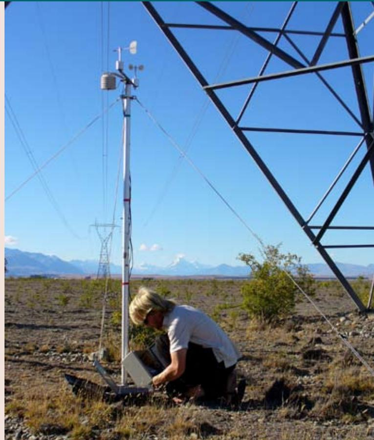
*Shane Rodwell downloads data from a portable meteorological monitoring station near Twizel during the power transmission line survey. Mt Cook is in the distance. [Photo: Steve Le Gal, NIWA]*
