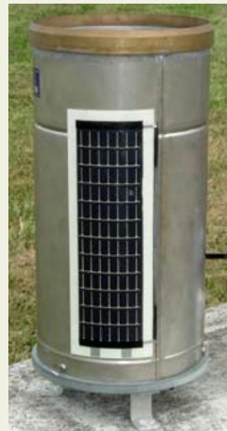
*NIWA's upgraded Rain Intensity Gauge showing the new flexible 'wrap around' solar panel. [Photo: Mike Hodkin, NIWA]*
