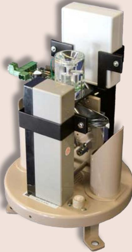
*The new SRIG, designed by NIWA Instrument Systems, provides simultaneous measurement of both total rainfall and rain intensity by one instrument – a major advance in rainfall measurement instrumentation. [Photo: Dave Gibb, NIWA]*
