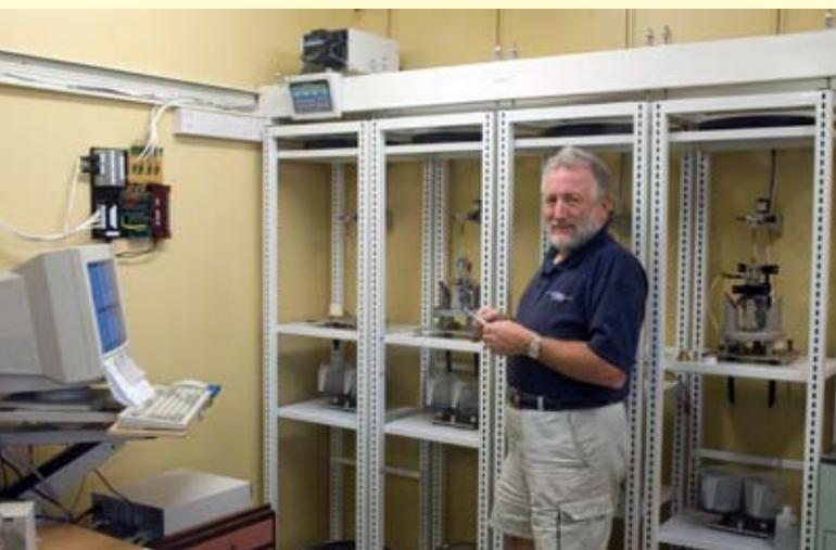
*Dave Gibb runs our upgraded calibration system for tipping bucket rain gauges. The system measures overall accuracy and other aspects of gauge performance including variations in individual tip capacity, the rain rate at which the calibration was performed, and the reed switch closure period. [Photo: Jeremy Bulleid, NIWA]*
