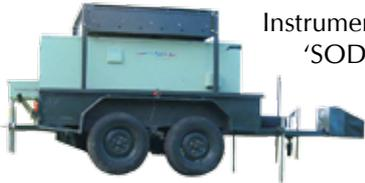
This self contained unit houses all of the control, communications, and power electronics. It is easy to set up and relocate, so can be used to quickly assess conditions at different positions within a proposed wind farm site. What's more, the analysis systems of the SODAR derive wind statistics and other information not readily available from conventional wind measurement technologies.
