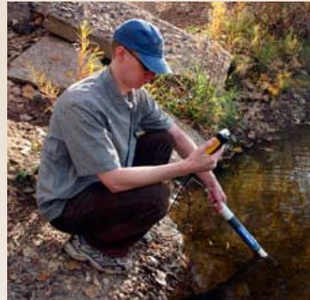
sensors in a hand-held wand, and a rugged pocket-sized display unit. Uses include: surface water-ground water interaction, stream restoration, wastewater effluent and stormwater runoff monitoring, dredging operations, low-flow sampling, and aquaculture.
