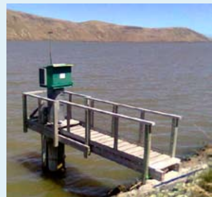
Looking seaward at Lake Forsyth. The monitoring station is solar-powered (solar panels visible on top & side of the station). [Photo: Marty Flanagan, NIWA]
