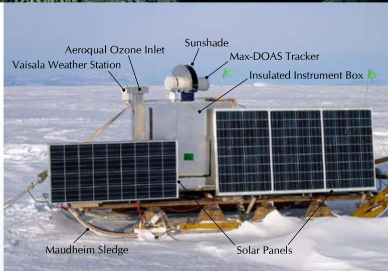
*The prototype MAX-DOAS instrument built at NIWA Lauder. This year the team used a diesel generator to supplement the solar panels since the instrument must be kept running at all times to avoid freezing. Next year, they hope to add a small wind turbine instead. Logistical support by Antarctica New Zealand is gratefully acknowledged. [Photo: Tim Hay, NIWA/Canterbury University]*
