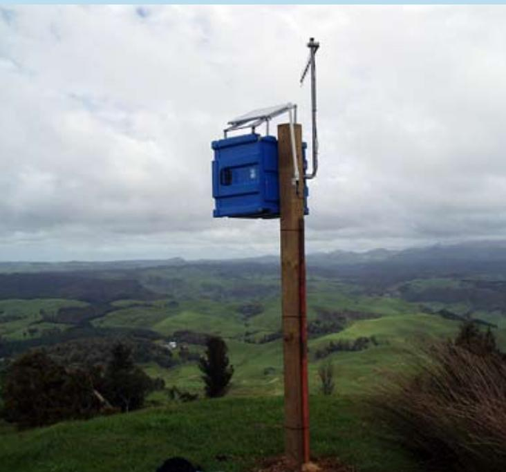
*The entire system – battery, solar regulator, and two modems – fits in a small box which can be easily fixed to a fence post. The equipment pictured enables NIWA's Marokopa water level measuring site to 'talk' to the Tuahu repeater site, Waikato. [Photo: Richard Keightley, NIWA]*
