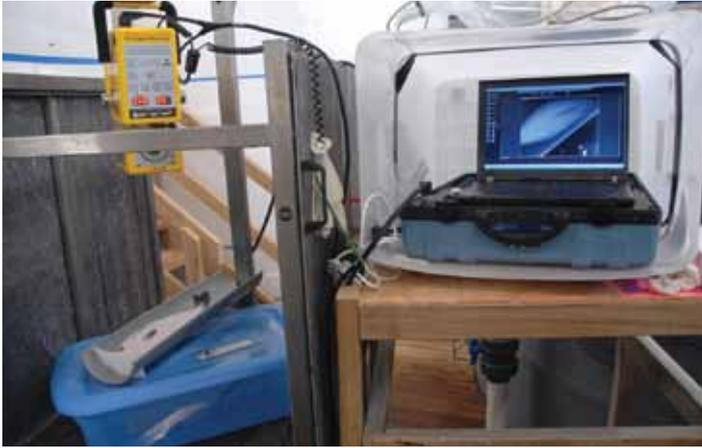
X-ray imaging equipment set-up.
