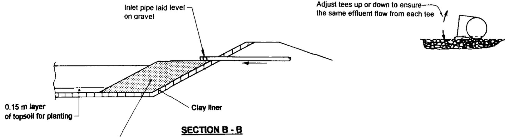
Unplanted splash pad, 65/40 mm clean hard gravel, no fines, 0.1 m above water level. Rotten rock or rock which crushes or weathers easily is not suitable
