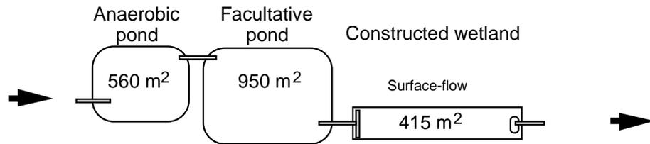
*Addition of a small surface-flow constructed wetland will provide basic buffering of flow and water quality*
