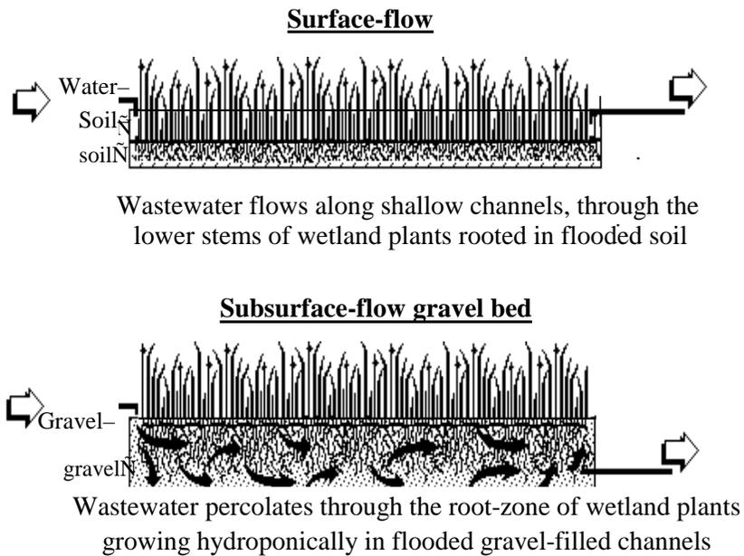
**Figure 1: Basic constructed wetland designs**
