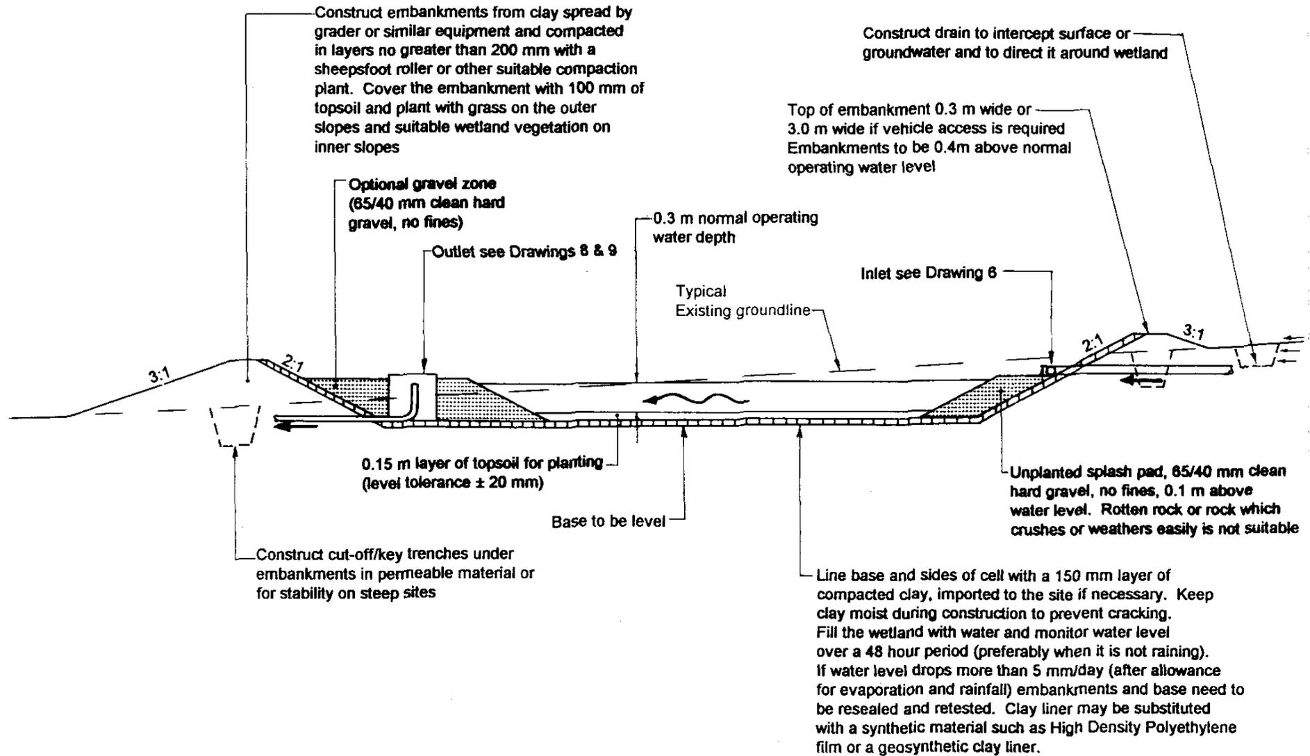
**Drawing 4: Surface-flow wetland channel—cross section**
