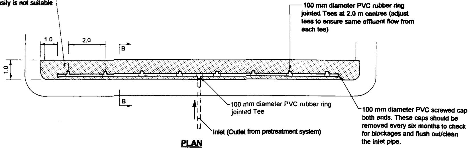
**Drawing 7: Alternative inlet structure using timber supports**
