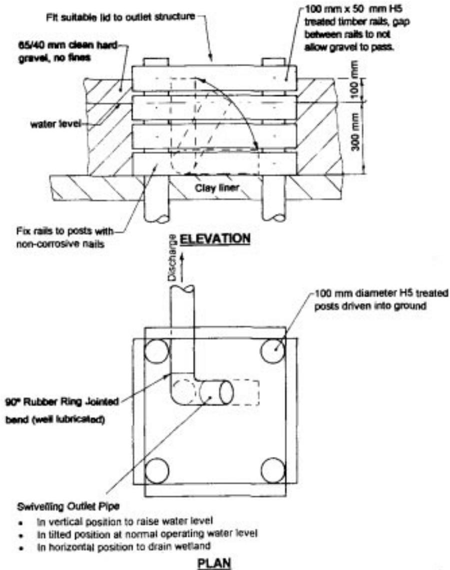
**Drawing 10: Alternative outlet structure for gravel-beds greater than 10 m in width.**
