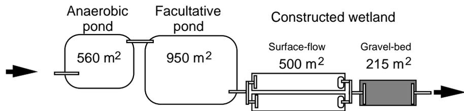
*Addition of a combined surface-flow and gravel-bed constructed wetland will provide a moderate level of treatment and buffering of flow and water quality*
