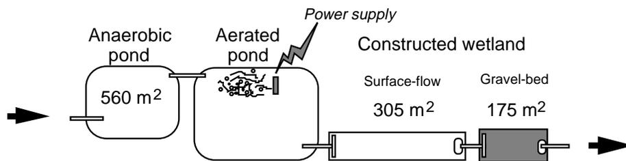
*Addition of a constructed wetland in association with aerated second pond will provide a high level of treatment. The constructed wetland will, in particular, enhance suspended solids, total nitrogen, and faecal coliform removal from aerated pond systems*
