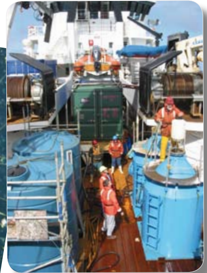
Preparation for release: the deck of RV Tangaroa with the iron tanks on the left and the \text{SF}_6 tracer tanks on the right.
