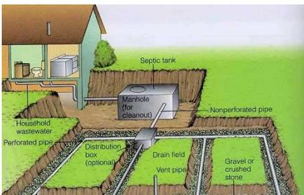
**Figure 1: Conventional septic tank system**
