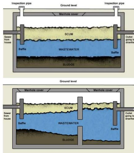
**Figure 2: Single and dual chambered septic tank**
