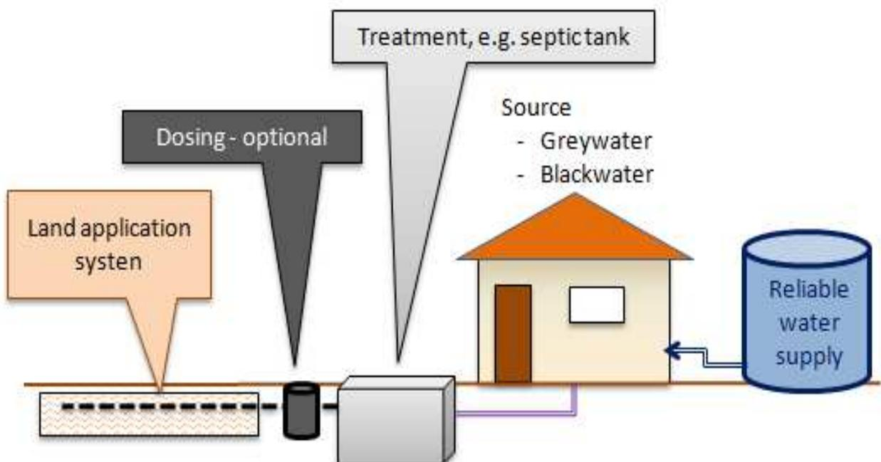
Figure 2: Typical two chamber septic tank for treatment of household blackwater. An outlet filter is recommended to reduce outflow of solids. Further treatment and safe discharge of the effluent is still required after the septic tank.
