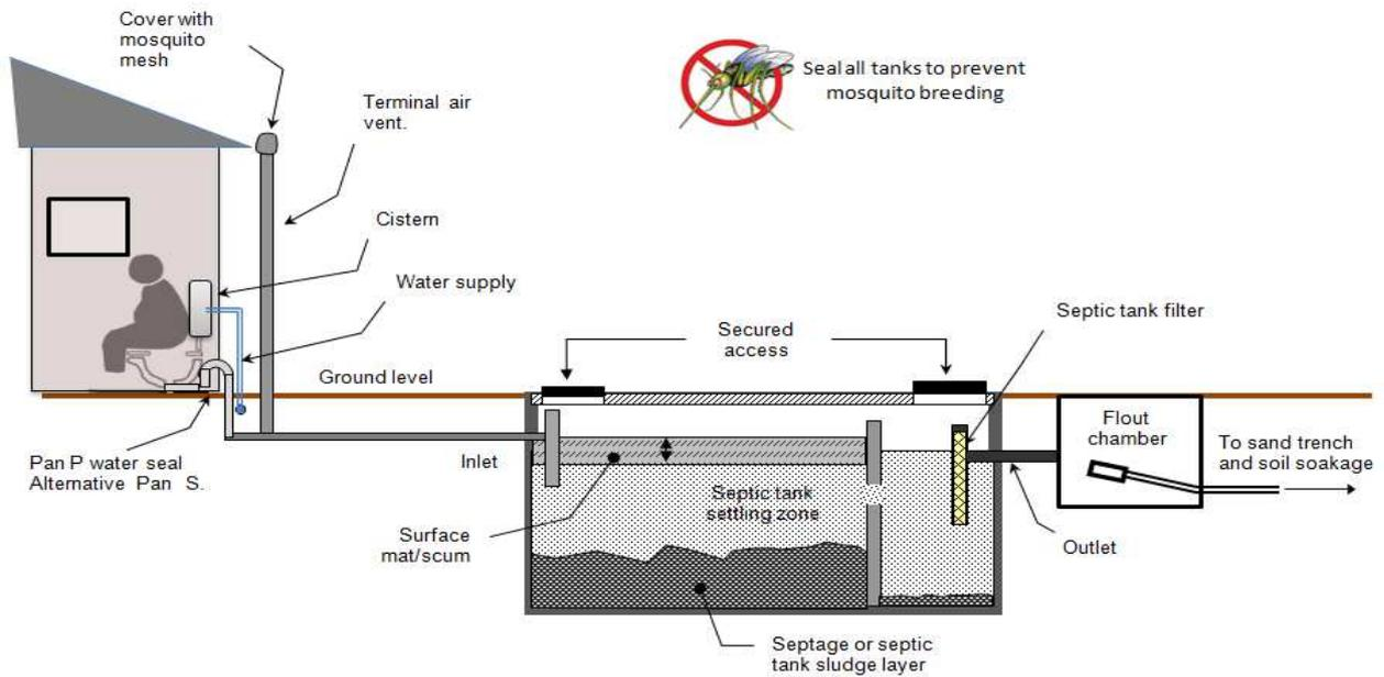
Figure 3: Typical two chamber septic tank configuration.
