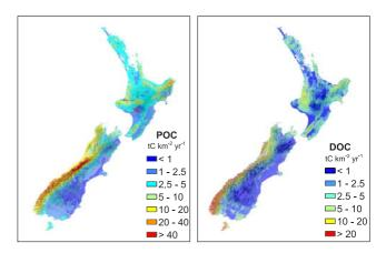
**Figure 2.** Particulate and dissolved organic carbon yields spatially distributed across New Zealand based on data for 47 and 44 stations, respectively. POC yields were estimated by applying a power-model that used mean annual precipitation and an adjustment for cells containing highly erodible terrain. DOC yields were estimated by applying a log-linear model that used mean annual precipitation, mean annual solar radiation, mean annual temperature, and slope.
