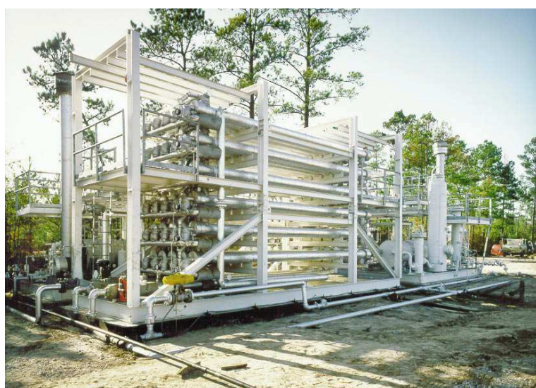
Figure 4.4.22 – Image and schematic of membrane based CO 2 removal plant
