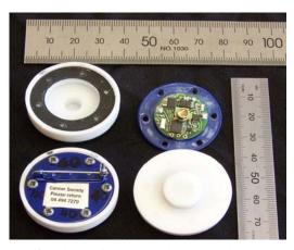
**Figure 1.** Electronic UV dosimeter badges + PTFE diffuser cap.
