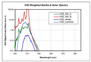
**Figure 3.** Spectra weighted by the action spectrum for erythema (upper panel) and vitamin D production (lower panel) from sunbeds compared with sunlight.
