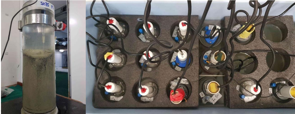
Figure 4-12: Experimental work: Oxygen probe measurements (left) and respiration experiments (right).
