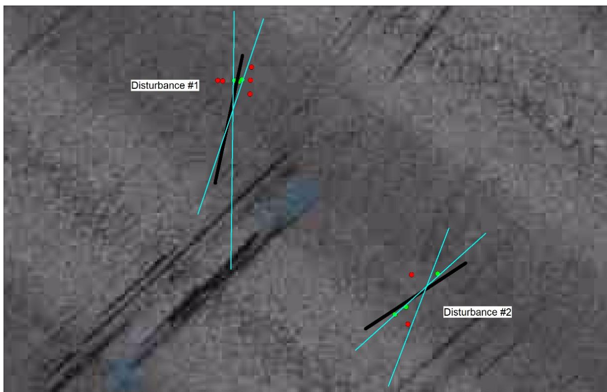
Figure 4-18: Beam trawl disturbance sites. Blue lines=DTIS tows before and after; black line=repeated beam trawl lines; green dot=multicorer inside line; red dot=multicorer outside line. Dark black “lines” are artefacts of MBES data.
