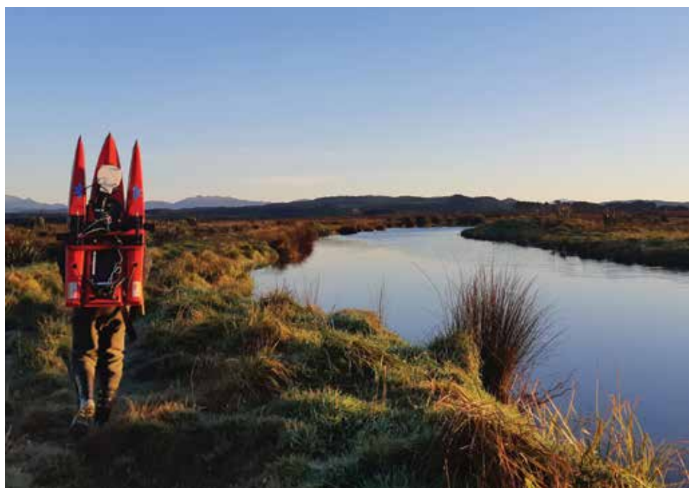
The remotely controlled Q1250 is not only more accurate than traditional methods for gauging river flow, it is also significantly safer. [Elliot Bowie]
