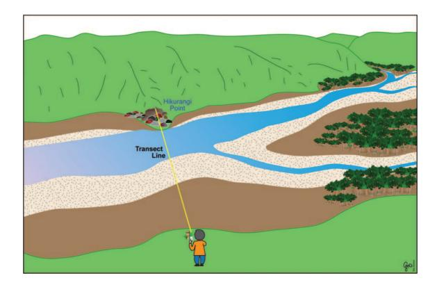
The transect (yellow line) starts at the benchmark and is lined up with Hikurangi Point on the north side of the harbour. The compass bearing along the transect is 338° magnetic.
