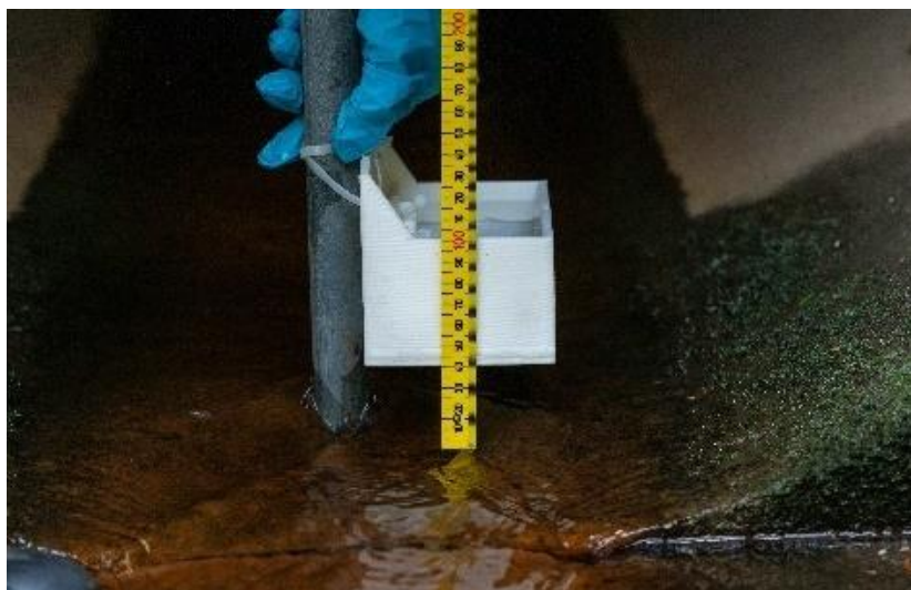
Figure 6: Installing trough on an adjustable pipe and measuring deployment height.
