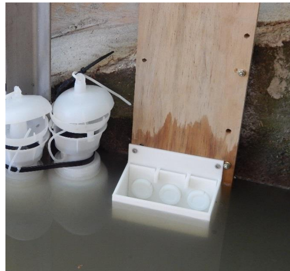
Figure 4: DGT trough holder mounted to (a) extendable pipe inside a stormwater pipe for a temporary installation and (b) timber bolted to stormwater outlet wing-wall for a more permanent deployment location.
