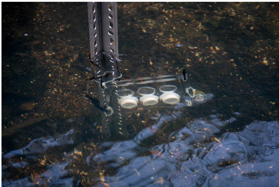
Figure 5: Deployment steps showing (a) DGTs contained within acrylic plate (b) with temperature recorder attached and (c) and plate attached to waratah.
