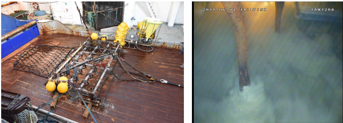
SCIP on deck, and a shot on the seafloor with the tynes digging into the sediment.
