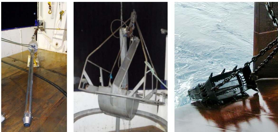
Figure 3. Left: Short gravity corer (1.6 m long barrel). Middle: Van Veen Grab. Right: Rock dredge.
