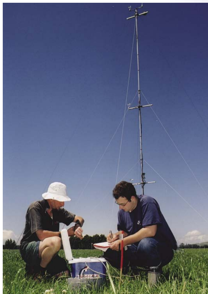
Tony Bromley and Paul Wilson with equipment to measure CO 2 fluxes from the soil surface.
