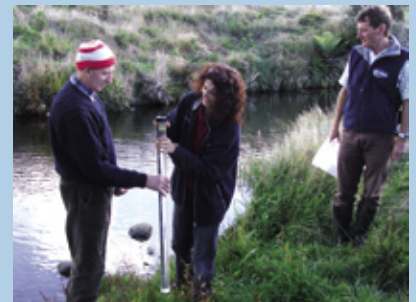
Steph Parkyn shows a Waitete landowner how to measure water clarity in a community stream restoration project.
