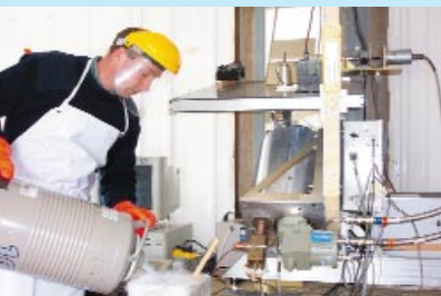
Mike Kotcamp calibrating the ozone microwave radiometer at Lauder.
