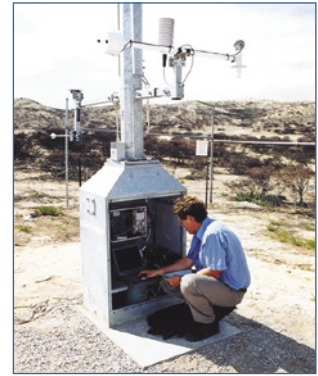
AMS hydrographer Gary Bruecher at one of the nineteen automatic weather stations around Western Australia using Unidata loggers.
