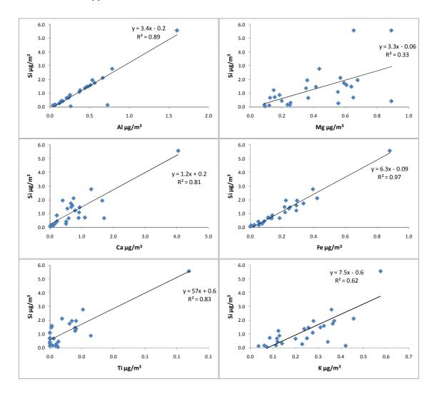
Figure 4.2: Linear regression of elements to Si based on measured elemental concentrations at Awatoto
