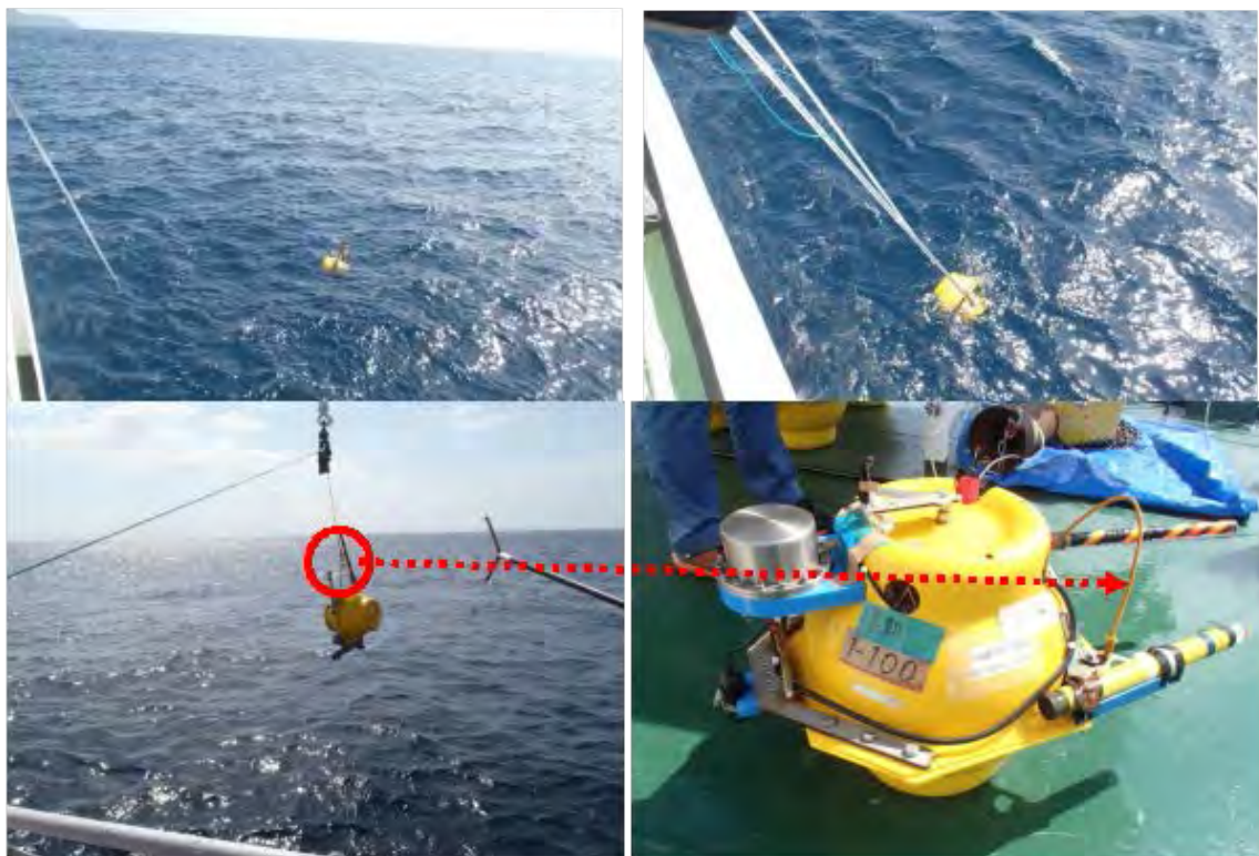
Figure 3.3 OBS Recovery. Anchors detach from the glass sphere assembly by means of electrolysis when recovered, thus allowing instrument to rise to sea surface. The instrument rotates so that the external transponder-side is down and strobe-side up. Strobe and radio-beacon attached to instrument to assist with recovery.
