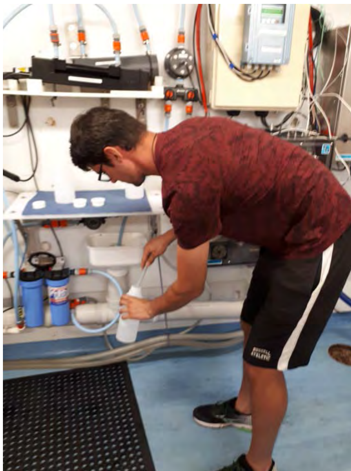
Figure 2.8 Filling sample bottles using the underway water sampling system.
