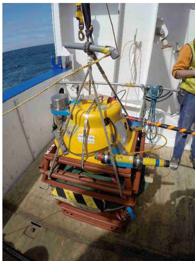
Figure 2.5 OBS at the Cutaway ready for deployment. Note rope sling through the anchor frame and quick release system comprising a PVC pipe (attached to a pull rope) as a peg through sling loop.
