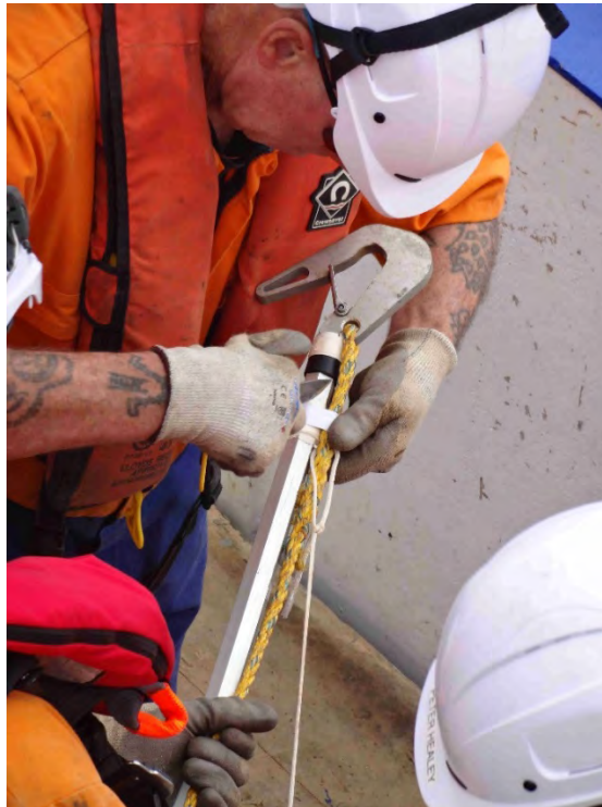
Figure 2.7 Preparation of detachable hook on pole. Hook is attached to a hoist rope on the A-frame winch and a tag line.
