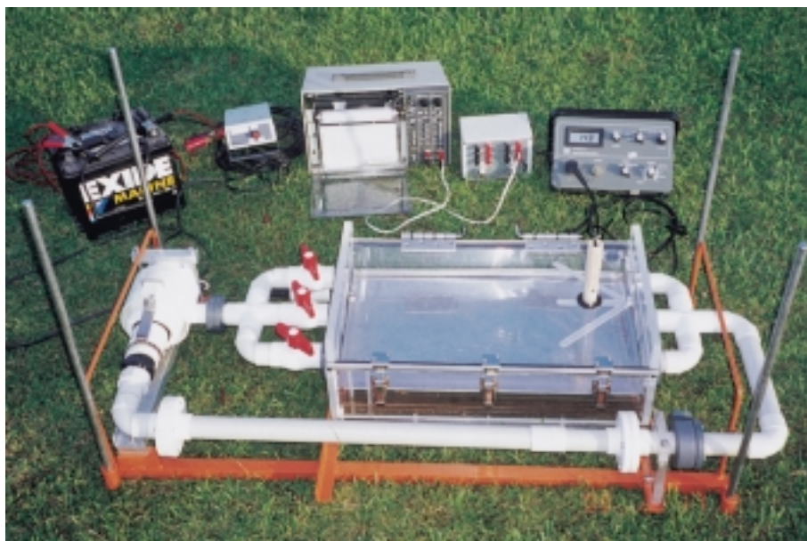
Figure 12: Benthic respirometer on adjustable legs. The submersible pump is mounted on the left end and dissolved oxygen probe is insert through a port on the lid of the main chamber. An in-line electromagnetic flow meter (not shown) can be inserted in the return flow line (foreground). Behind the respirometer are the (from left): 12-V DC marine grade battery to power the pump, voltage controller, chart recorder, scale expander and dissolved oxygen meter. The overhead lighting system is not shown (see Figure 13).
