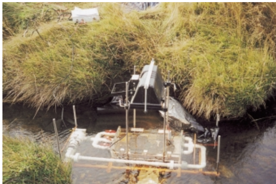
Figure 13: Undertaking P_{max} measurements with the benthic respirometer. A 1500 Watt lamp is mounted over the respirometer to provide standardised, high light for incubations. The light is power by a generator on the bank (out of photo).
