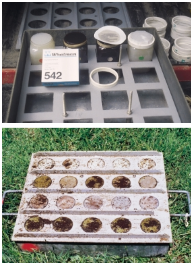
Figure 11: Steel-tray nutrient-diffusing substrate sampler. Top: sampler without the lid attached showing the internal frame of the sampler. The four agar-filled jars at the rear show stages in securing the filter-paper colonisation surfaces to the jars. The phosphorus-enriched agar jars are dark in colour. Bottom: nutrient-diffusing substrate sampler after incubation with the lid attached (the upstream end is marked with red paint on the left). Treatments from the far side are: control, nitrate + phosphate, phosphate, nitrate .
