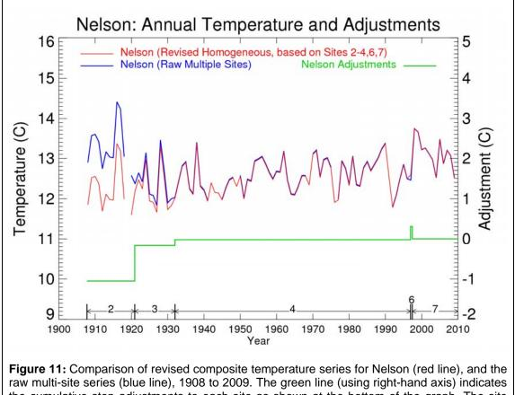
the cumulative step adjustments to each site as shown at the bottom of the graph. The site numbers and periods of record correspond to those listed in Table 1.
