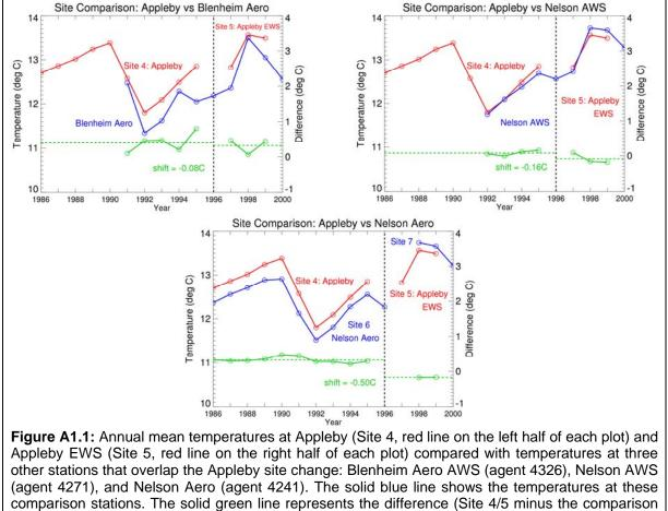
comparison stations. The solid green line represents the difference (Site 4/5 minus the comparison station) using the right-hand ordinate scale. The horizontal dashed green line is the average difference before and after the site change. The year of the site change, 1996, is indicated by the vertical dashed line. The lower plot uses the raw data from Nelson Aero (both Sites 6 and 7) without adjustment, with the year of the site change (1997) removed.
