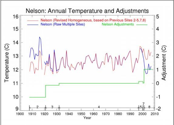
**Figure A1.5:** Comparison of revised composite temperature series for Nelson from 1908 to 2007 (red line), based on the previous site selection, with the raw multi-site series (blue line). The green line (using right-hand axis) indicates the cumulative step adjustments to each site as shown at the bottom of the graph. The site numbers and periods of record correspond to those listed in Table A1.1.
