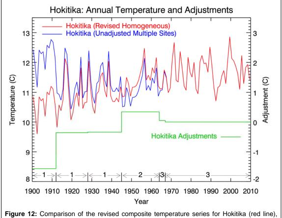
**Figure 12:** Comparison of the revised composite temperature series for Hokitika (red line), with an unadjusted composite series (blue line) from 1900 to 2009. Numbers near the bottom of the plot denote the site labels of Table 1, with vertical lines marking the time periods over which each site contributes to the composite series. The green line (using right-hand ordinate scale) indicates the adjustment for each period.
