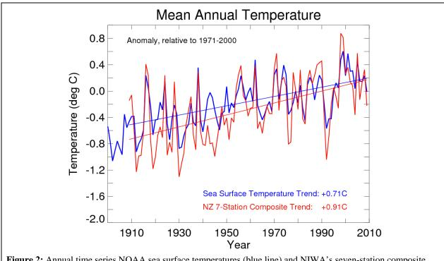
**Figure 2:** Annual time series NOAA sea surface temperatures (blue line) and NIWA's seven-station composite series (red line), expressed as anomalies relative to the 1971-2000 climatological average. Linear trends over the period 1909-2009, in °C/century, are noted under the graph.
