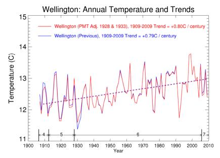
**Figure A3.2:** Composite series of annual mean air temperatures for Wellington (red line) from 1900 to 2009. The adjustments in 1928 and 1933 were diagnosed by the penalised maximal t test, as described in the text. The blue line shows the previous NIWA composite series for Wellington. The dashed lines show the fitted linear trends from 1909 to 2009. Wellington site labels from Table 1 are displayed at the bottom of the plot.
