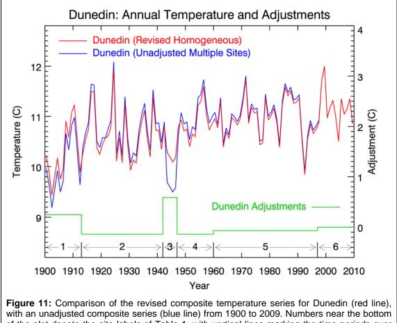
with an unadjusted composite series (blue line) from 1900 to 2009. Numbers near the bottom of the plot denote the site labels of Table 1, with vertical lines marking the time periods over which each site contributes to the composite series. The green line (using right-hand ordinate scale) indicates the adjustment for each period.
