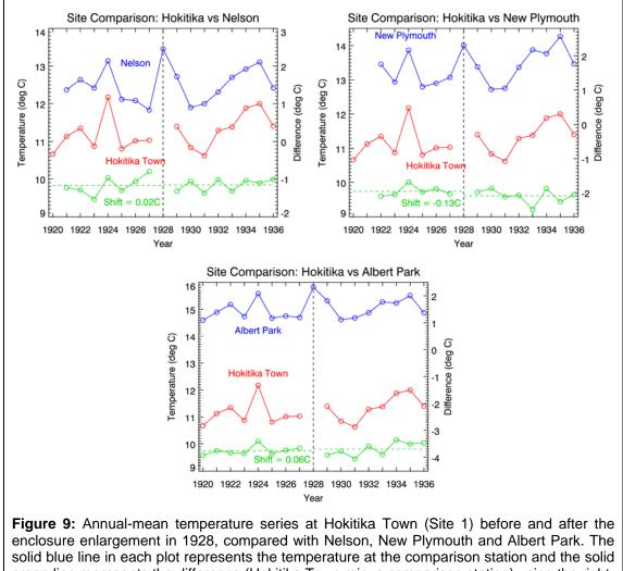
enclosure enlargement in 1928, compared with Nelson, New Plymouth and Albert Park. The solid blue line in each plot represents the temperature at the comparison station and the solid green line represents the difference (Hokitika Town minus comparison station) using the right-hand ordinate scale. The year of the change, 1928, is indicated by a vertical dashed line. The mean differences for the periods before and after the change are indicated by dashed green lines.
