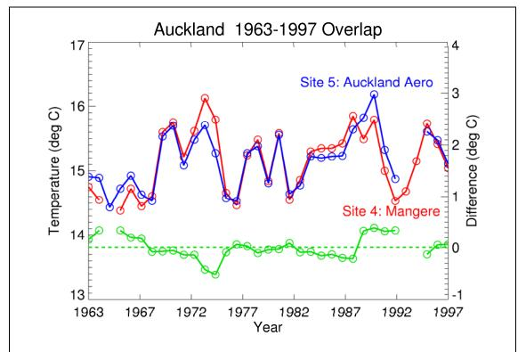
**Figure 3:** Annual mean temperature series for Mangere (Site 4, agent 1945, red line) and Auckland Aero AWS (Site 5, agent 1962, blue line) from 1963 to 1997. The annual difference, Site 5 minus Site 4, is plotted by the green solid line, using the right-hand ordinate scale, and the mean annual difference is shown, in green, by the dashed line.
