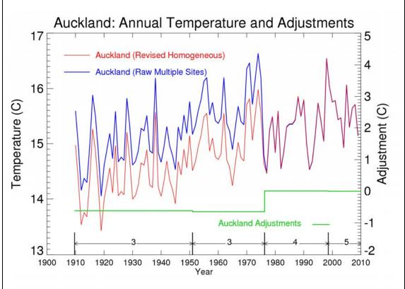
**Figure 8:** Comparison of the revised composite temperature series for Auckland from 1910 to 2009 (red line), with the raw multi-site series (Sites 3-5, blue line). The green line (using right-hand axis) indicates the cumulative step adjustments to each site as shown at the bottom of the graph, and corresponds to the adjustments in the right-hand column of Table 1.
