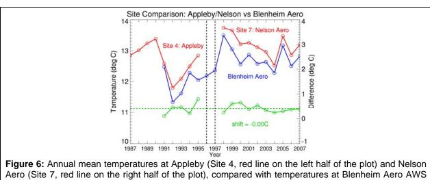
Aero (Site 7, red line on the right half of the plot), compared with temperatures at Blenheim Aero AWS (blue line). The solid green line represents the difference (Site 4/7 minus Blenheim) using the right-hand ordinate scale. The horizontal dashed green line is the average difference before and after the site change. The years of the site changes, 1996 (for Appleby) and 1997 (for Nelson Aero), are indicated by the vertical dashed lines.
