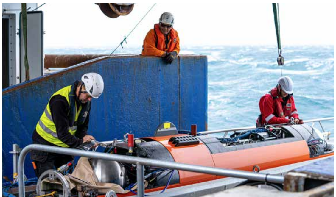
Technicians reprogramme Rán as the AUV prepares for its next mapping mission off the Kaikōura coast. (Lana Young)
