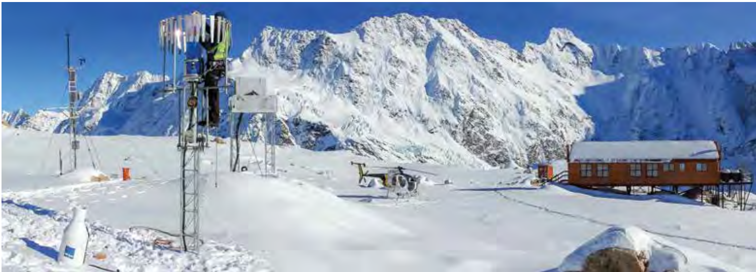
The Mueller Hut weather station, 1800m above sea level. One of 11 stations NIWA manages to gather high-elevation meteorological data such as snow density. (Jeremy Rutherford)
