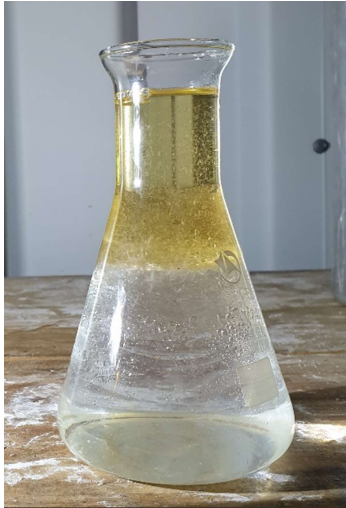
Figure 5: A sample of freshly distilled Totara essential oil separating from the water phase.
