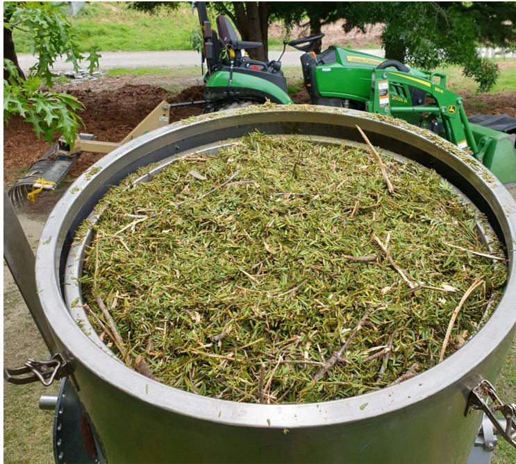
Figure 4: Chipped Totara foliage loaded into the batch still, ready for essential oil extraction.
