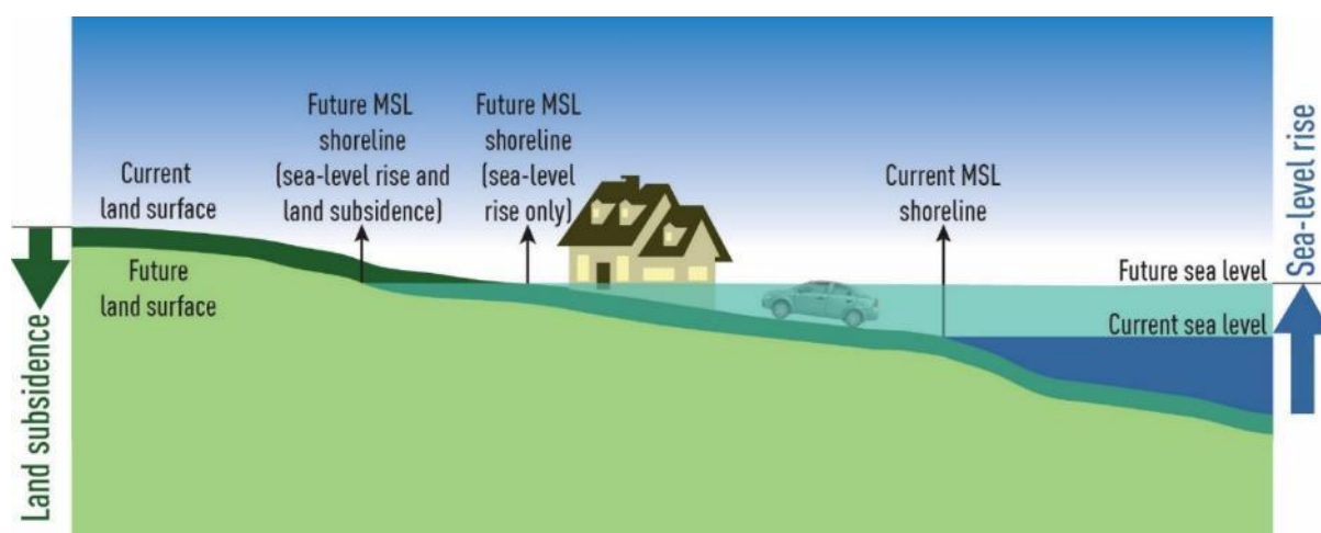
Figure 8-1: Difference in mean sea level (MSL) shoreline between absolute and local (relative) SLR where land subsidence occurs.
