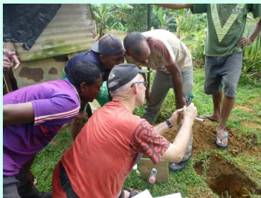
Soil testing to determine soil capability for drainage
