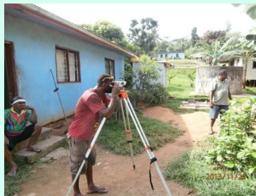
Checking ground levels and gradients
