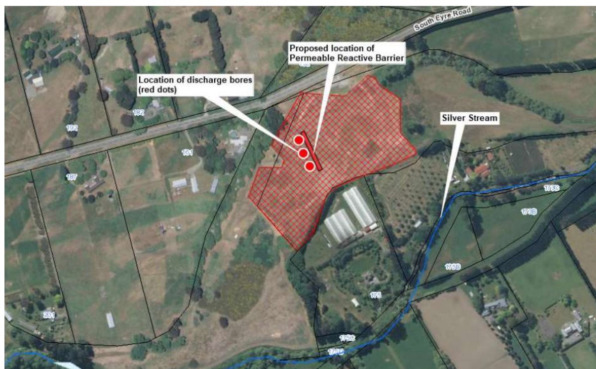
Figure 4-4: Proposed PBR site location and location of bores for the discharge of sodium chloride tracer solution to groundwater. The site is within Silverstream Reserve, Clarkville in the Waimakariri District (ESR, in Duke 2017).
